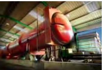
At 17m long and 3m diameter the new treatment vessel is capable of treating over 40m³ in one charge.
