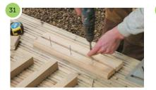
Starting from the centre mark the position of the spindles on the handrail. For easier fitting start the screws in position on the rail before attaching the spindles.
