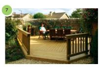
If there is not room below your damp proof course to build a deck without excavation, consider a free standing deck, leaving room between the house and deck to prevent water standing or splashing against the wall.
