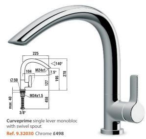
Min 2.0 bar pressure required 140° swivel spout Mounting hole size ∅ 35mm
