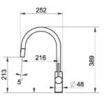
Oxygen single lever monobloc mixer with swivel spout and pull-out rinse
