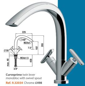
Min 2.0 bar pressure required 140° swivel spout Mounting hole size Ø 35mm
