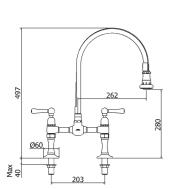
**Steam Valve** Deck-mounted bridge mixer with swivel spout and lever controls
