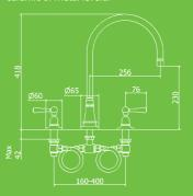
**Steam Valve** Three hole mixer with swivel
