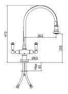
**Steam Valve** One hole bridge mixer with swivel spout and lever controls
