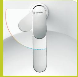
The Linfa uses an innovative energy saving cartridge. This means the lever when central only dispenses cold water not mixed as others taps do. This prevents firing the water heater each time you turn on the tap.
