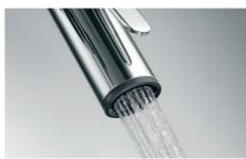
The professional spray on the Highflex can be used while the swivel spout is in use. Pressing lightly on the adjustment lever on the spray head activates the needle spray. As soon as the adjustment lever is released, the water comes out of the swivel spout again.
