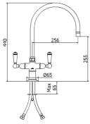
Steam Valve Monobloc with swivel spout and lever controls Ref. 1021BS Brushed Stainless Steel £436 Ref. 1021PS Polished Stainless Steel £498
