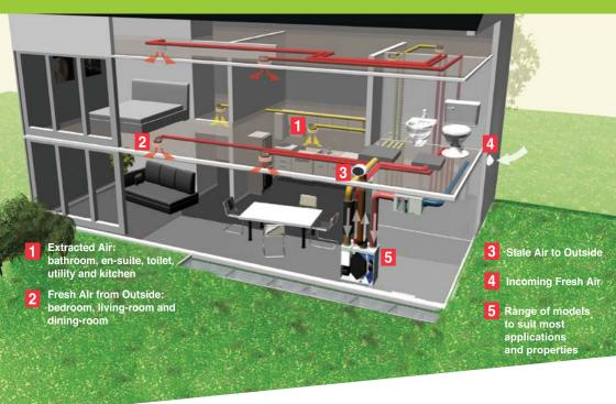
Heat recovery systems draw in fresh air from outside, while at the same time extracting stale air from within the house. As the fresh air and stale air travel through the counter-flow heat exchanger inside the unit, the thermal energy from the used air is recycled and used to heat the fresh incoming air. Basically as a heat pump, it recycles 80% of the thermal energy from the air.
