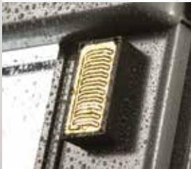
Rain Sensor for auto closing
