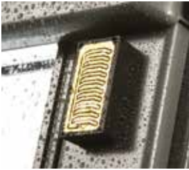
Rain Sensor for auto closing
